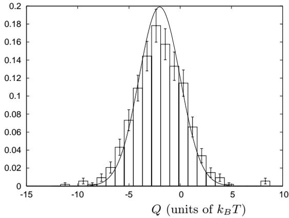
FIG. 3: Histogram of the heat exchanged by the colloidal particle with the environment, with  $v = 1 \mu\text{m/s}$ , and  $t = 0.5 \text{ s} \gg \tau$ , as given by eq. (3). The line correspond to the expected PDF as given by eq. (20), with no adjustable parameter.
